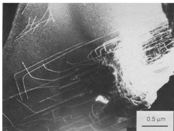
Fig. 15. TEM micrograph of HPAIN deformed 2.1% at 5 \times 10^{-6} \text{ s}^{-1} , 1650°C. Dislocation loops made of straight segments in non-basal planes. Long segments are parallel to the trace of the basal plane and have a nearly pure screw character. Weak beam conditions, 2 g. g: \bar{2}110 , foil normal and beam direction: [10\bar{1}0] .
